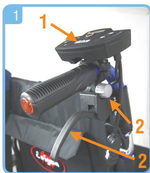
Figure 1: 1. Controller, 2. Inner Knob, 3. Trigger.
